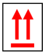
FIGURE 4 Label which indicates correct orientation of package during shipping.
