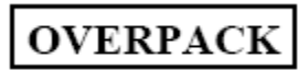
FIGURE 6 Marking which indicates an overpack is used and inner packages comply with regulations.
